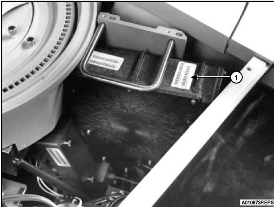
Fig 5. The photometer assembly. A section of the reaction carousel is adjacent.
